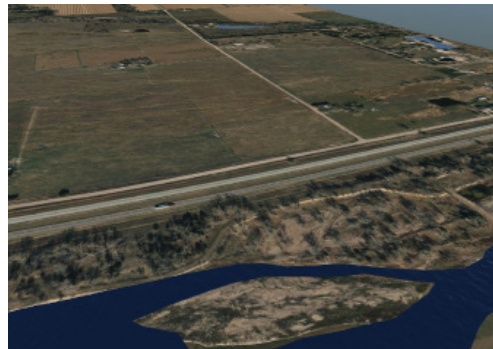
Pictured: Renderings of the Kearney diversion channel, pictured before (top) and after (bottom). The Kearney diversion channel is estimated at 200-ft. bottom width and 5,350-ft. in length.
