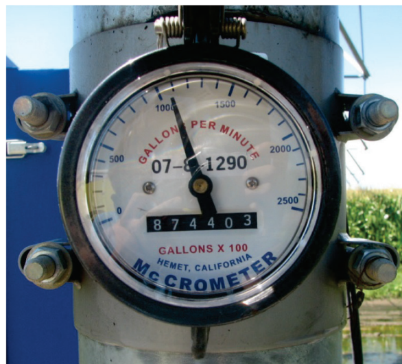
Figure J-2. Impeller flow meter commonly used to monitor the water flow rate in an irrigation pipeline.
